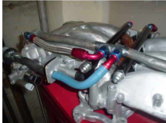
Figure 3 — Idle air plumbed with AN hose fittings
