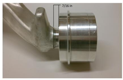
Press the bracket onto the new bushing. Be sure to press it in with the same orientation as the stock bushing so it will mount properly to the chassis. You may need to press the bushing onto the arm a bit more to get the bolt holes for the bracket to line up.
