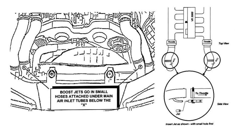
**NOTE** THE BOOST JETS SUPPLIED IN THIS KIT ARE SIZED TO PRODUCE A BOOST LEVEL OF 12 TO 13.5 LBS. THE BOOST MUST BE CHECKED WITH AN ACCURATE GAUGE TO DETERMINE WHETHER YOUR BOOST PRESSURE IS IN THIS RANGE AFTER INSTALLING THE UPGRADE. IF BOOST IS LOWER, FULL POWER MAY BE LIMITED. IF BOOST IS TO HIGH, "PING" OR DETONATION MAY OCCUR (THIS MUST BE AVOIDED!). SPECIAL JETS CAN BE ORDERED TO CORRECT EITHER CONDITION.
