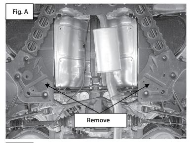
1.) Remove the 2 bolts + 1 nut shown in Fig. A to take off the undercover tray. (Both sides)
