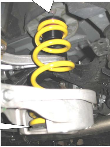
Use the original spring support at the bottom end of the spring.
