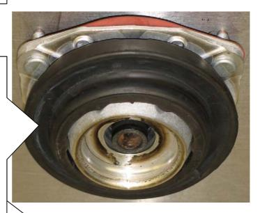
After you have completed installation of the suspension, check the clearance of the tyres to the front suspension strut. The minimum clearance at the narrowest point is 5 mm and must, where necessary, be provided using commercially available, Technical Inspectorate (German TUEV) approved spacers.
