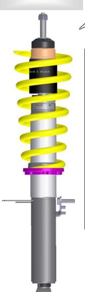
Install the factory supporting bearing without the standard bump stop and fix it with the supplied stop nut. Tightening torque for the piston rod nut is 35 Nm (26 ft-lb). The strut unit has to be installed according to manufacturers recommended settings regarding tightening torque and fixing specifications.
