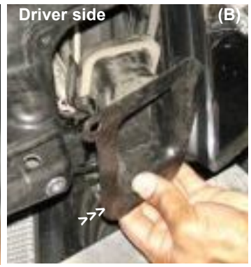
Figure 23 Remove the plastic clips from the front air scoops which are located in front of the passenger side (A) and the driver side (B) cross member.
