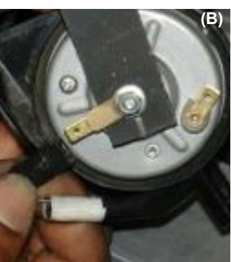
Figure 28 The first horn is aligned and attached to the new bracket, the copper connectors are re-attached prior to securing it with the nut (A). The copper connector is re-attached and the electrical wires are reconnected as shown above (B).
