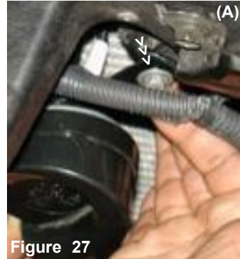
Figure 27 The 10mm bolt on the driver side horn bracket is removed (A). The electrical wires are disconnected from the driver side horn, the nut is also removed in order to separate the horn from the bracket (B).
