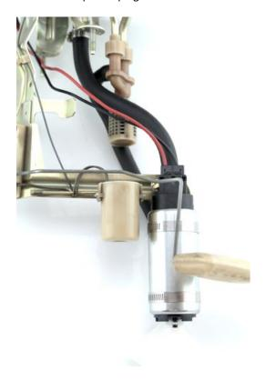
6 – reinstall the assembly into the fuel tank and attach a length of hose to the outlet of the pump assembly allowing it to drain into a fuel safe container and prime the fuel pump assembly
