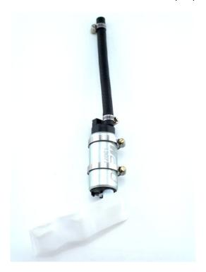
4 – install the DW pump to the lower extension of the fuel pump assembly. Take care to position the fuel sock in the same location as the OE fuel sock that was removed
