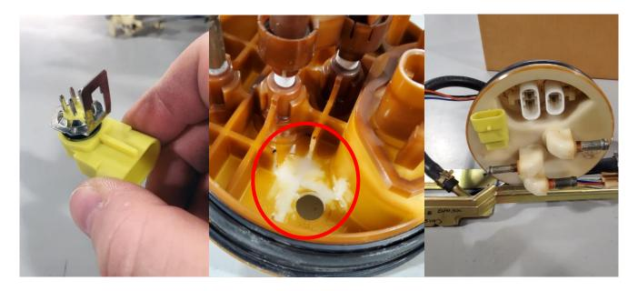
6 – The factory fuel pump power and ground wires can be removed or covered so they will not short on the module. Attach the supplied Brushless pump harness to the bulkhead and the DW440 pump.
