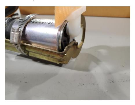
4 – Install the supplied fuel safe submersible rubber hose between the pump and the module, use the two supplied adjustable hose clamps to secure the hose in place. The supplied hose is 4 inches long, it may be cut down to fit as needed.
