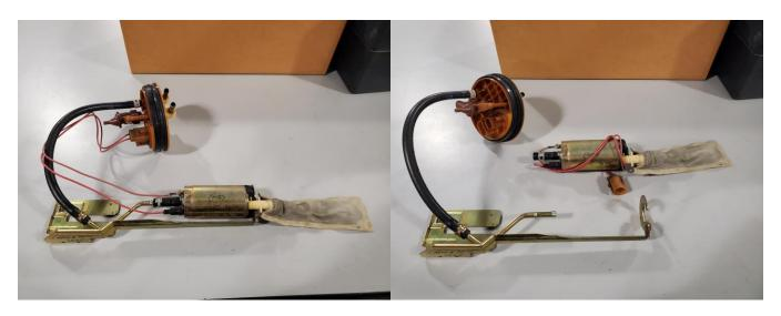
2 – Attach the supplied filter sock to the bottom of the DW Brushless fuel pump, secure the filter sock with the included star washer, this can often be difficult to install, it can be made easier by using a socket to push evenly on the edges of the washer. Install the supplied submersible fuel safe rubber hose and secure with one of the supplied 5/16" adjustable hose clamps.
