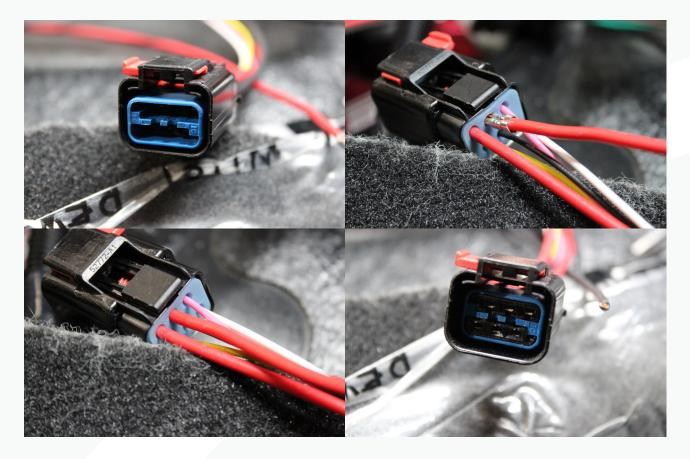
93. Put a 180-degree bend in the green and brown wires and then bundle the group of wires together. Starting from the OEM loom, wrap the wiring with electrical tape up to the T. Then place a section of electrical tape near the 180-degree bend to hold the other bundle in place.
