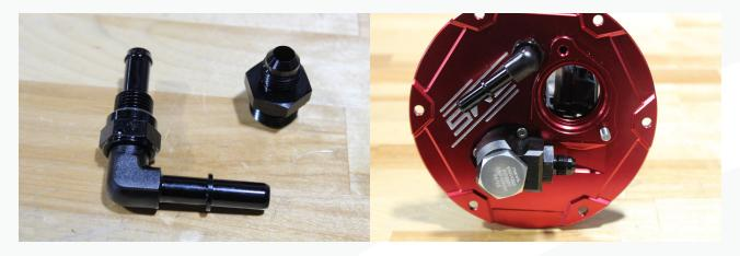
22. Grab the fuel pump, fuel pump grommet, and fuel pump fitting. Lubricate the grommet inside and out, then install it into the fitting. Then lubricate the O-ring and install the fitting in the open port.
