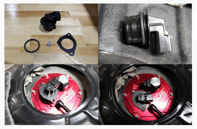
76. Install the white quick disconnect clip removed early onto the top hat fitting. Reconnect the factory fuel line to the now return port.
