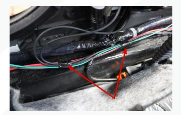
102. Stretch out the 3/8" split loom from the relay towards the front of the car and up into the dash area, mark it, then add 24" so it reaches into the battery compartment.
