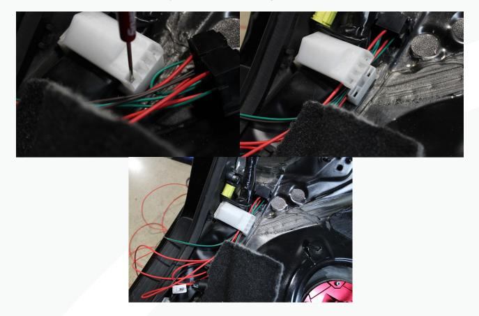
88. Feed the long unterminated ends of the green and brown wires through the same grommet as shown.
