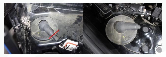
108. Feed the wires up through the hole into the battery compartment. Then while holding the grommet, feed the wires and loom through the grommet at click the grommet back in place.
