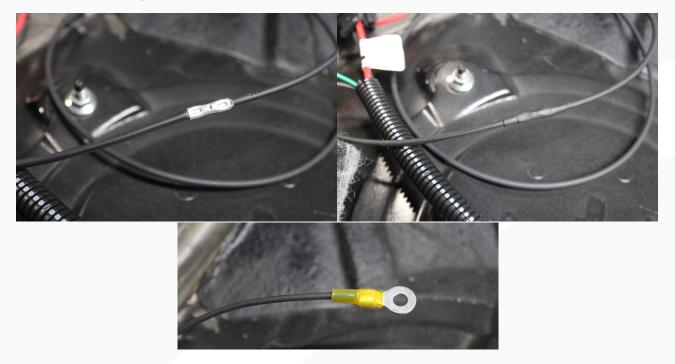
99. Route the (2) red wires, (2) ground wires and green/brown Hobb switch wires through the vehicle harness retainers along the sill up to the b-pillar.
