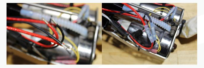
43. If you are working with a previously installed system, cut the existing zip ties securing the wires together. Then using two new zip ties, re-secure the wires with the added red wire in two locations shown below.
