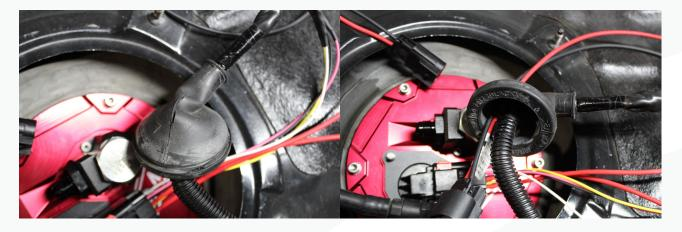
82. Locate the two relay harnesses. The one on the left is the primary pump harness, the one on the left if the add on harness.
