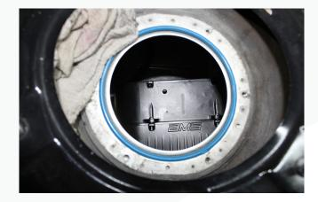
66. Lay out the level sensor mount, level sensor bracket, and M5 bolt. Apply a small amount of red Loctite to the bolt and install the level sensor mount to the basket as shown below.
