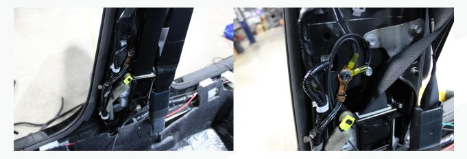
101. Apply two pieces of tape to the group of wires near the B-pillar as shown below
