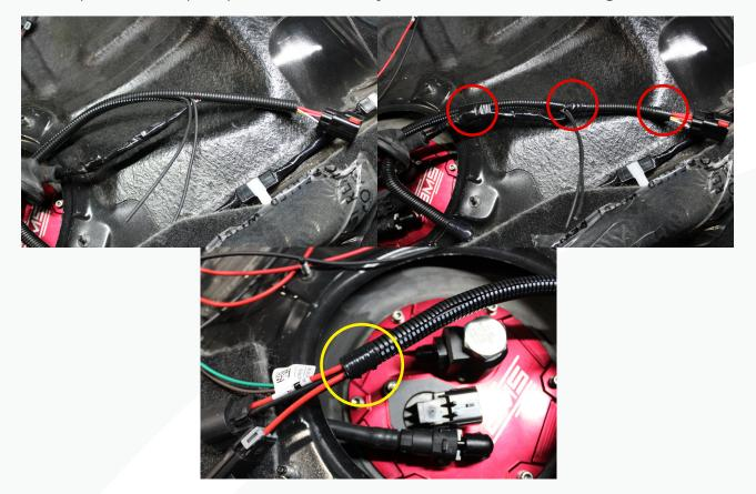
95. Strip the two black wires and crimp on the provided eyelet terminals. Use a heat gun on the heat shrink.
