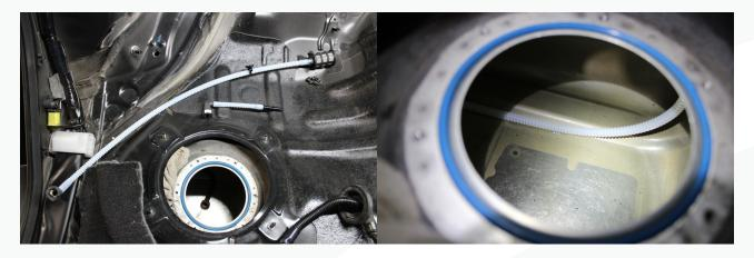
62. Install the short siphon hose into the black hose connection inside the tank.
