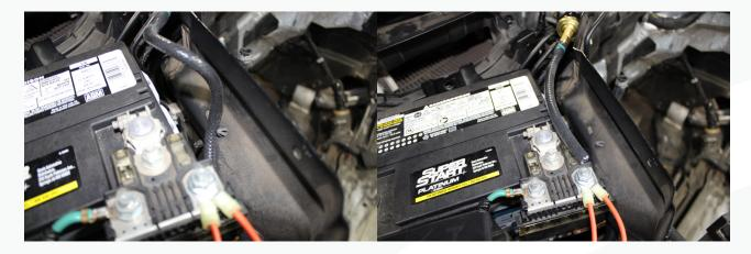
117. Install the straight barb fitting with a clamp and point the other end through the hole.
