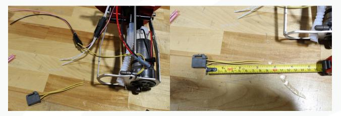
33. For the Q50/60, trim about an inch off the provided AMS harness. Using a wire stripper, prepare the wires to make two butt connections. Polarity does not matter in this step.
