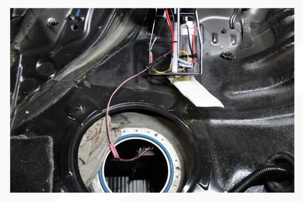
70. Before installing the fuel pump assembly, check that the corrugated hose routes just underneath the level sensor but does not contact it.
