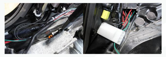
104. Secure the loom closed with electrical tape right before the (2) ground wire leaves the loom at the B pillar.
