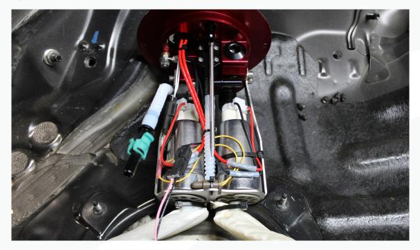
72. While lowering the fuel pump assembly into position, make the two hose connections on the siphon block.
