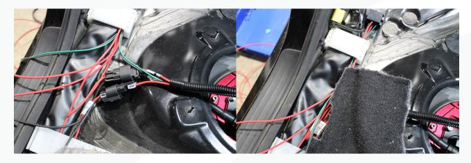
97. Locate the (2) 32" unterminated black wire, ring terminal, butt connector, and a 1 1/4" piece of 3/16 heat shrink. Strip the end of the black wire on the end of the 2-pin connector and both ends of the unterminated black wire.
