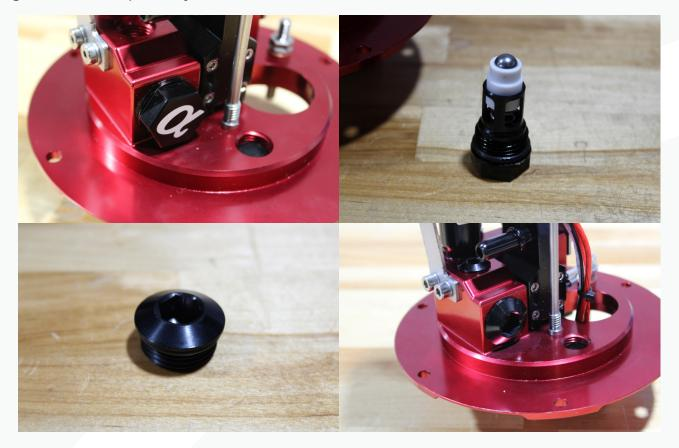
20. On the top of the top hat, remove the quick connect fitting and 6AN plug.
