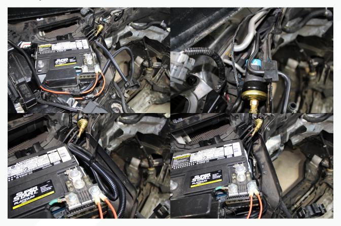
115. Locate the 5mm hose, clamps, and barb fittings. Install one clamp to the hose and then secure it to the hobb switch.
