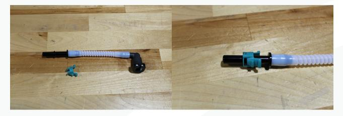
54. Gather the larger 3/8 siphon hose, 3/8 90 degree quick connect fitting, siphon strainer, magnet, zip tie and cinch clamp #14.5.
