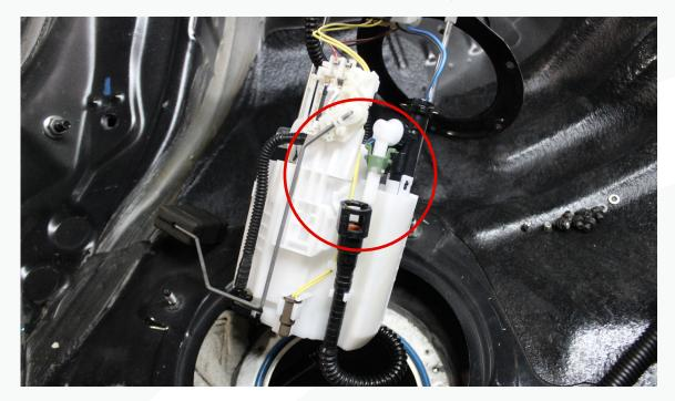
10. On the driver's side, remove the top hat/level sender assembly just like you did for the passenger side. Set it aside for now.
