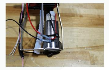
29. Loosely install ground wire eyelet to the stud on the bottom of the top hat using the provided M6 nut and split washer in the orientation shown below to hold it temporarily.
