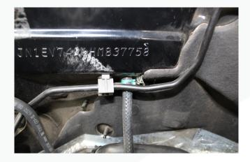
119. The other end of the hose needs to be connected to a boost source like the intake manifold. Some extra clamps and a tee fitting have been included to accomplish this.
