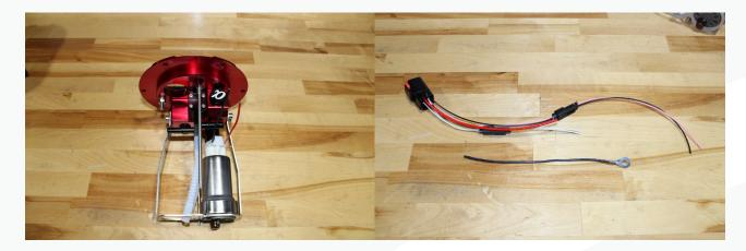
26. Place the large connector side of the harness through the opening in the top hat about an inch or so. Strip the end of the red wire of the harness about 3/8" from the end. Repeat on the fuel pump red and black wires along with the single black wire with eyelet.
