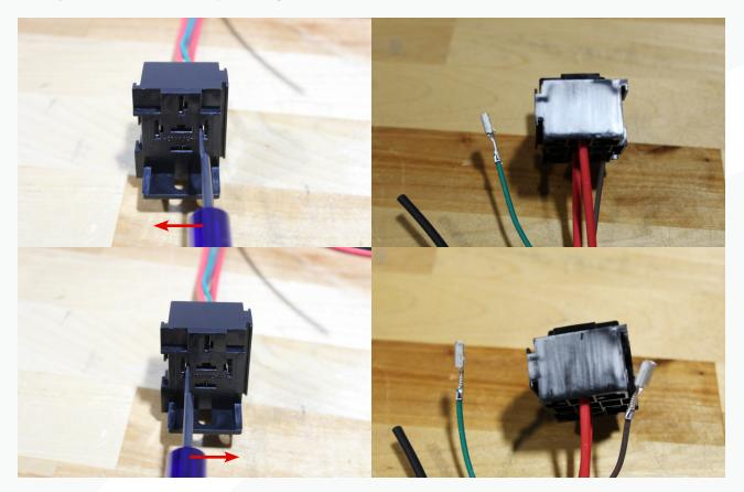
84. Attach the two relay holders together with the primary on the left and "add on" on the right.
