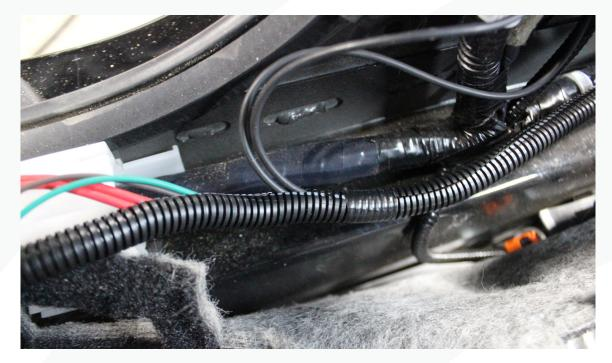
105. Continue feeding the harness in the loom. Once the whole harness has been loomed, feed it through the rest of the harness retainers along the sill.
