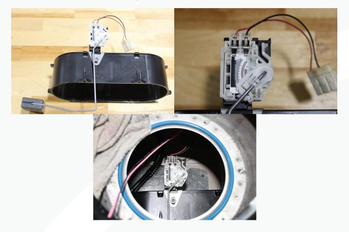
68. Position the basket so that the side with the level sensor is facing the back of the car. This should position the float just above the corrugated siphon line previously installed.
