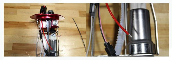
27. Using two blue butt connectors, match the colors red to red, black to black and crimp them using crimping pliers for insulated connectors.
