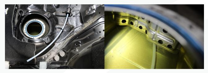
59. Push the open end of the hose onto the metal tube at the front of the tank.
