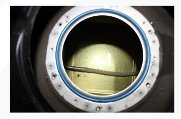
60. Reinstall the driver's side top hat and replace the O-ring if necessary. Then reinstall the connector and cover panel.
