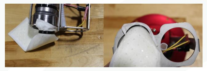
36. Using one zip tie, attach the white section of wire to the side of the hanger. Put retainer side of the zip tie on the inside as shown below.
