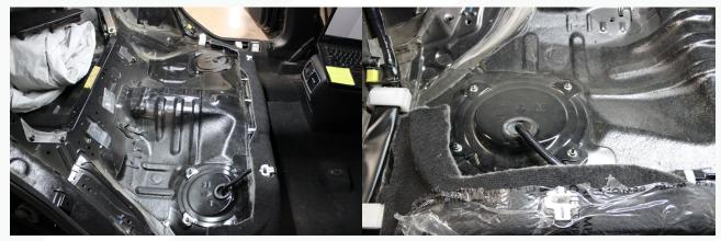
6. Remove the access panel and disconnect the fuel line quick disconnect and top hat electrical connector.
