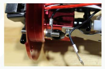
41. Run the ground wire with the rest of the wires on the connector, if necessary, trim the black ground wire so it is the same length as the red wire.
