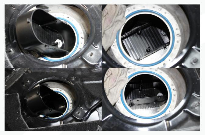
64. Loosely reinstall all the screws to hold the basket together. Then carefully snug them down until you feel resistance. DO NOT OVERTIGHTEN or you will strip the plastic.
