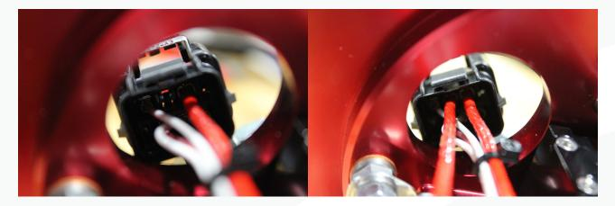
40. Remove the ground nut from the top hat and install the second ground wire. Position the two eyelets back-to-back and tighten the nut. Be sure to clock them down so they are almost touching the top hat.
