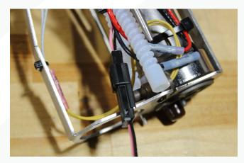
46. Cut off the OEM level sensor connector about an inch away from the connector.
