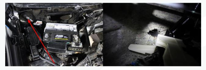
107. Trim the grommet indicated by the red line below just before it enlarges. This spot will fit tight on the loom to help prevent leaks.
