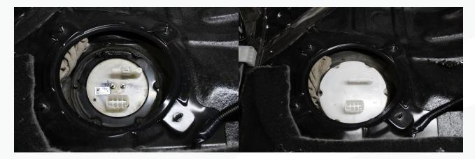
8. Carefully lift the fuel tank sending unit to not damage any of the corrugated tubing or wiring. Once you have it mostly out you will need to tip it back slightly to get past the level sender.
