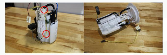
14. Push the level sensor retaining lock over and slide the sensor up and out.
