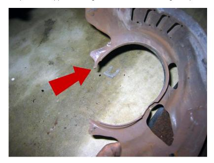
**Figure 2** – Cut factory dust shield at the front of the hub.
