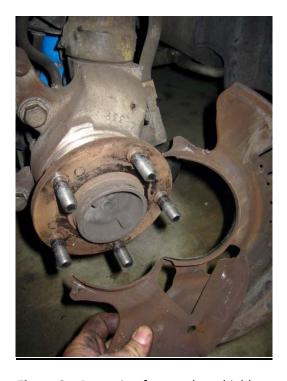
Figure 3 – Removing factory dust shield.
