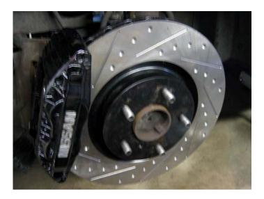
Figure 6 – 350Z track rotor kit installed.
