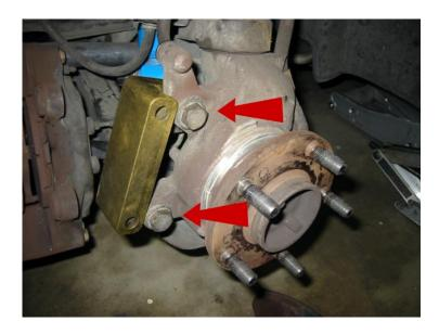
Figure 4 – Bolt adapter to spindle using OE caliper hardware
