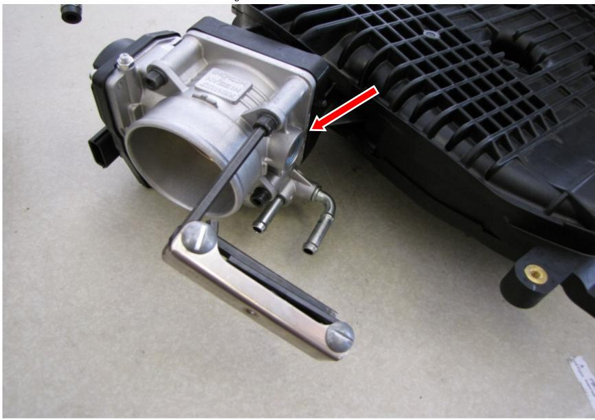
Remove the throttle bodies from the stock manifold using a 5mm Allen wrench and transfer the throttle bodies to the M370 manifold.
