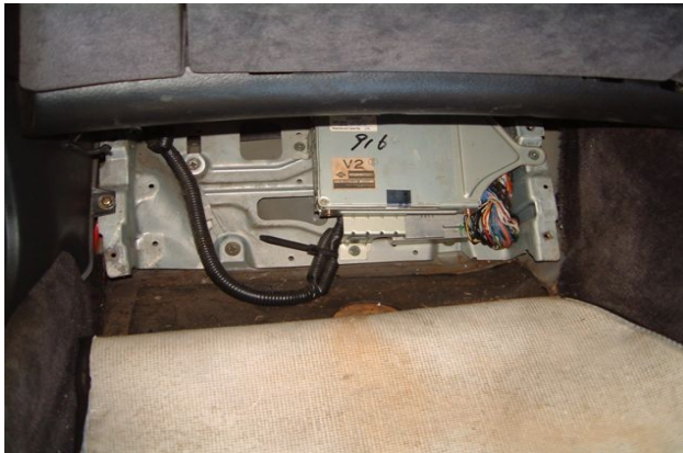
Figure 2 – Factory ECU Mounting Location with cover removed
